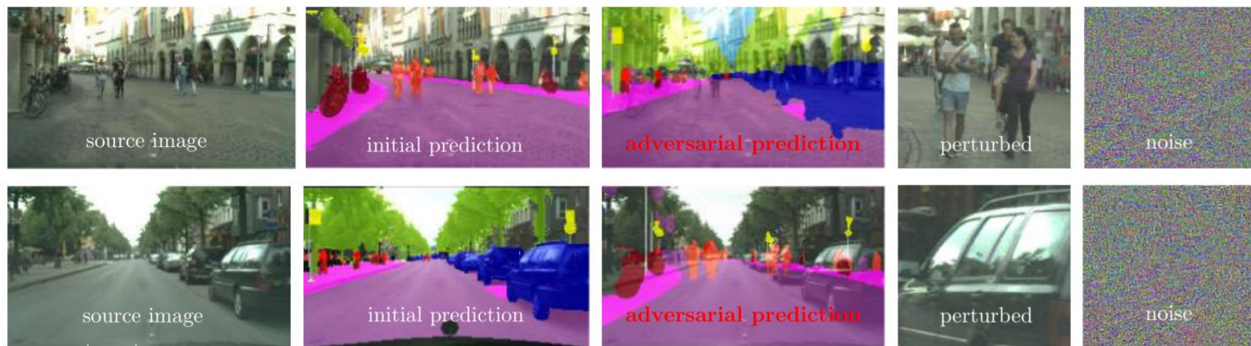
Figure 4: Targetted attack on a semantic segmentation system: switching target segmentation between two images from Cityscapes dataset [8]. The last two columns are respectively zoomed-in parts of the perturbed image and the adversarial perturbation added to the original one.
